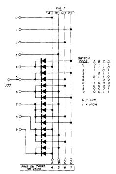
fig. 4. Alternative selector switch and diode matrix circuit.
